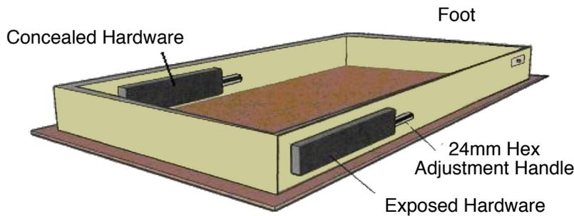
Install bed platform in a wall cabinet or between pier cabinets with a bridge.
