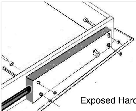
**Supplied countersink bushings are necessary to reduce stress when platform is in motion.**
