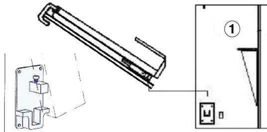
Lift door platform and bed frame on a 45° angle to clear all obstructions and lower the assembly into place with the square axels in the mount plate saddles in the cabinet.
