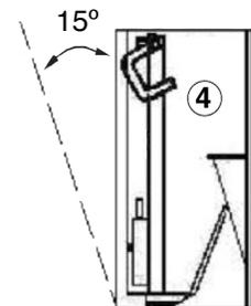
Open door to 15° and tighten tension sequentially, a few turns on one side and a few turns on the other until the door panel is balanced. The door panel is balanced when the door will stand at about 45° open. See FAQ page for detail.
