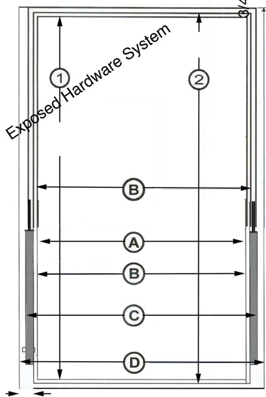
A 3/4" hardwood plywood cabinet back must be provided for cabinet integrity and attachment of the cabinet to a structural wall. The platform can weigh several hundred lbs, and will be in motion when opening or closing.
